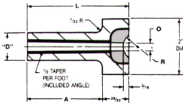
Made of MoldStar®150 material (Beryllium-free) with hardened 420 S.S. insert at nozzle seat area.
