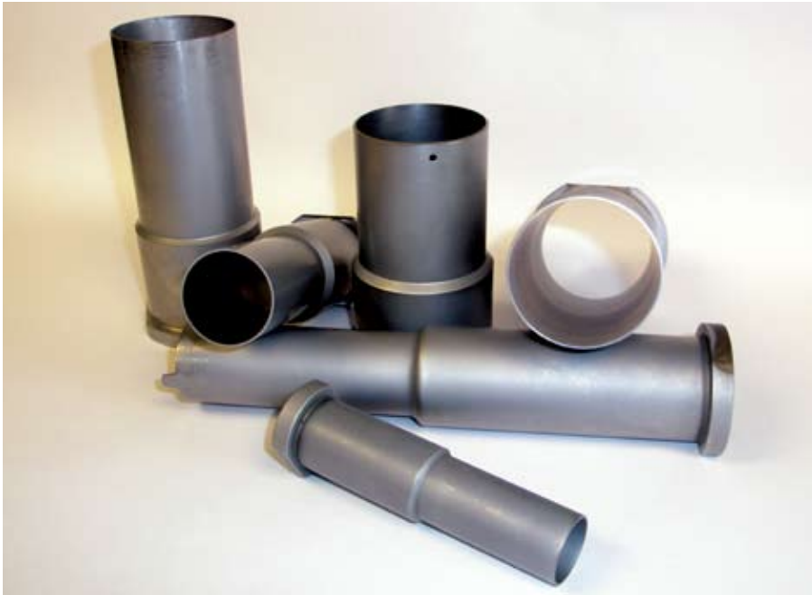
Custom sleeves made using aluminum bronze alloy that are TDC (thin dense chrome) coated to prevent galvanic reactions between tool steel inner core and plastic resin additives (also note "vent" or vacuum relief hole on standing sleeve on the right).
