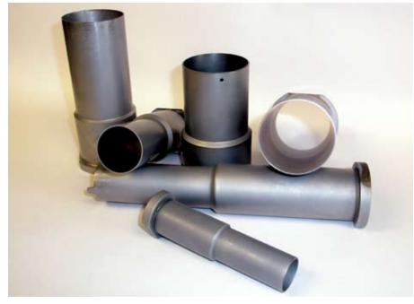
Custom sleeves made using alumimum bronze alloy that are TDC (thin dense chrome) coated to prevent galvanic reactions between tool steel inner core and plastic resin additives (also note "vent" or vacuum relief hole on standing sleeve on the right).
